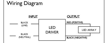
Input and Output use lead-wires. Lead-wires are 20AWG 80C/300V stranded copper
