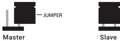
1. Select one receiver to be the master and install the jumper on one pin.
