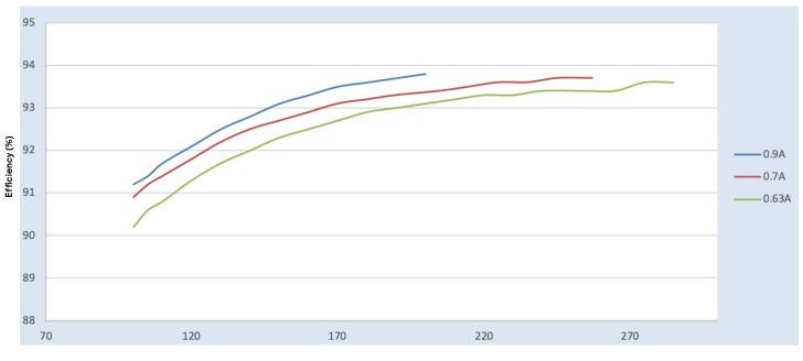
Efficiency Vs. Output Voltage at 347Vac
