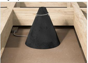
The FF109-200 is a cone-shaped intumescent enclosure which has been designed to help protect openings for **4**<sup>*n*</sup> **low profile LED downlight fixtures**. The high expansion and insulating properties of the material ensure that both, flame spread and heat transmission, are stopped for 60 minutes. The **flexible material** allows the cover to get rolled up for easy retrofit or new construction installation.
