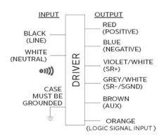
Input and output use lead-wires.
