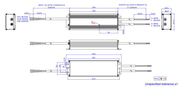
Note: The 2 DC output cables are connected in parallel internally because one AWG #18 wire can only carry 10A. Please connect the 2 red wires together and 2 black wires together in application, or ensure each cable carries same current.
