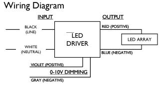
Input, Output and 0-10V Dimming use lead-wires. Lead-wires are 18AWG 105C/600V solid copper
