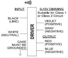
Input and output use lead- wires.
