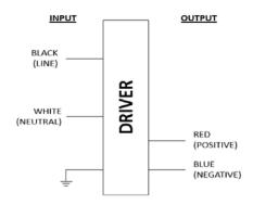
Input and output use lead-wires.
