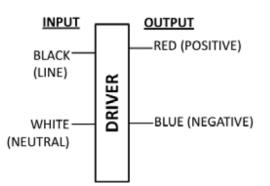
Input and output use lead wires.
