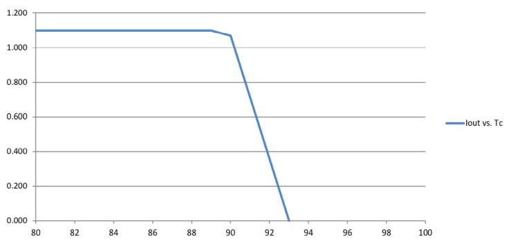
Note: There is ±5°C tolerance on the driver case temperature.
