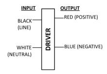
Input and output use lead wires.
