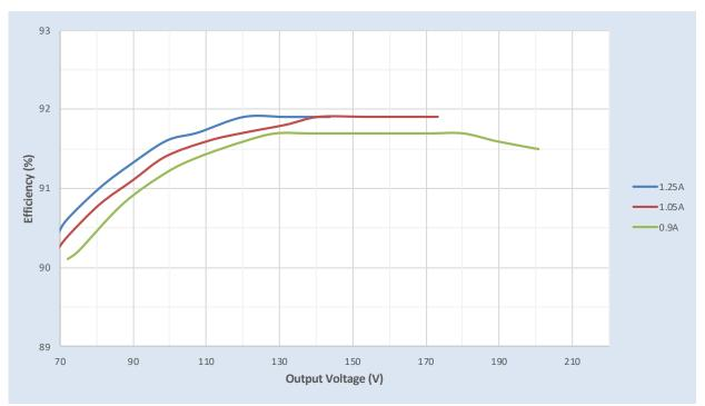
Efficiency Vs. Output Voltage at 277Vac
