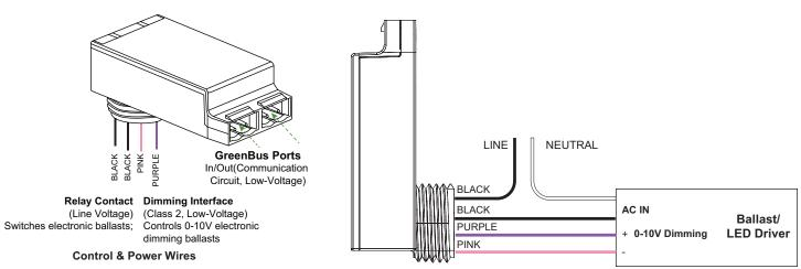
NOTE: Recommended relay switching capacity 120-347V, 300W max.
