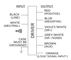
Input and output use lead-wires.
