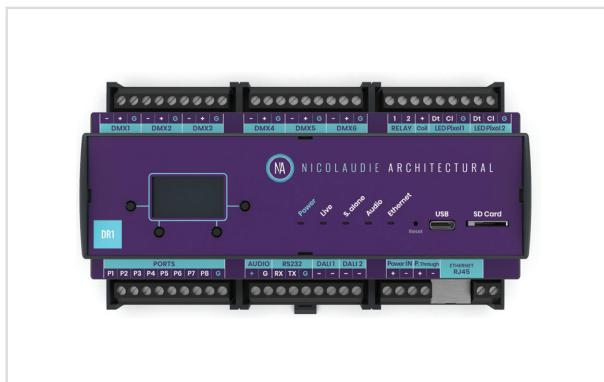
Designed for din-rail mounting, the DR1 is a strong and durable solution for fixed lighting installations. Up to 3072 channels (1024 RGB or 768 RGBW fixtures) can be controlled over several protocols: DMX 512, Art-Net or SACN, LED Pixel, DALI. Multiple controllers can be connected and synchronized for large-scale lighting installation.
