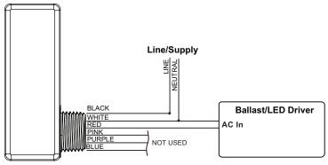
For a non-dimming fixture, cap off Pink, Purple, and Blue wire ends with UL Listed Wire Nut
