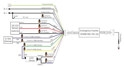
2. For luminaire with 0-10V LED driver, without using 0-10V dimmer (\* LED DRIVER INPUT POWER NOT GREATER THAN 80W) Emergency Inverter Dim+ (Green), Driver Dim- (Yellow) has to connect with LED driver DIM+ and DIM-
