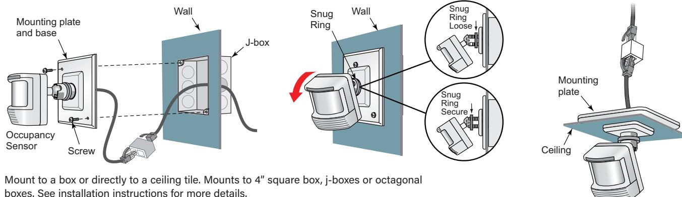
Mount to a box or directly to a ceiling tile. Mounts to 4" square box, j-boxes or octagonal boxes. See installation instructions for more details.
