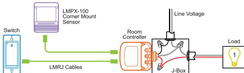
Plug DLM local network components together in any configuration using Cat 5e cables with RJ45 connectors.
