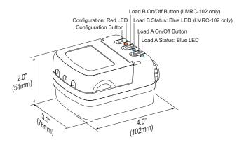
LMRC-100 Series Room Controllers include a 1/2" (12.7mm) threaded nipple and locking ring.
