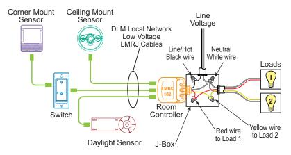
Plug DLM local network components together in any configuration using Cat 5e cables with RJ45 connectors.
