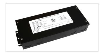
PowerFactor Dimmable Drivers provide smooth, stable, and efficient dimming capability for LED lighting. They are compatible with many models of Triac, ELV, MLV, forward and reverse phase dimmers, and on/off switches. All PowerFactor multi-tap models, and wattages up to 24V/96W, are Class 2 compliant, making them safe and inspection-ready.
