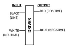
Input and output use lead wires.
