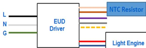
Figure 34: Adding NTC Thermistor for External OTP
