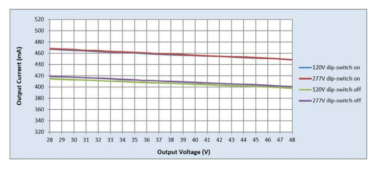
When designing LED board, please consider LED voltage increases due to cold temperature, forward voltage tolerance and aging to make sure LED voltage is always below 48V. Recommended typical LED voltage at room temperature 43V or below.
