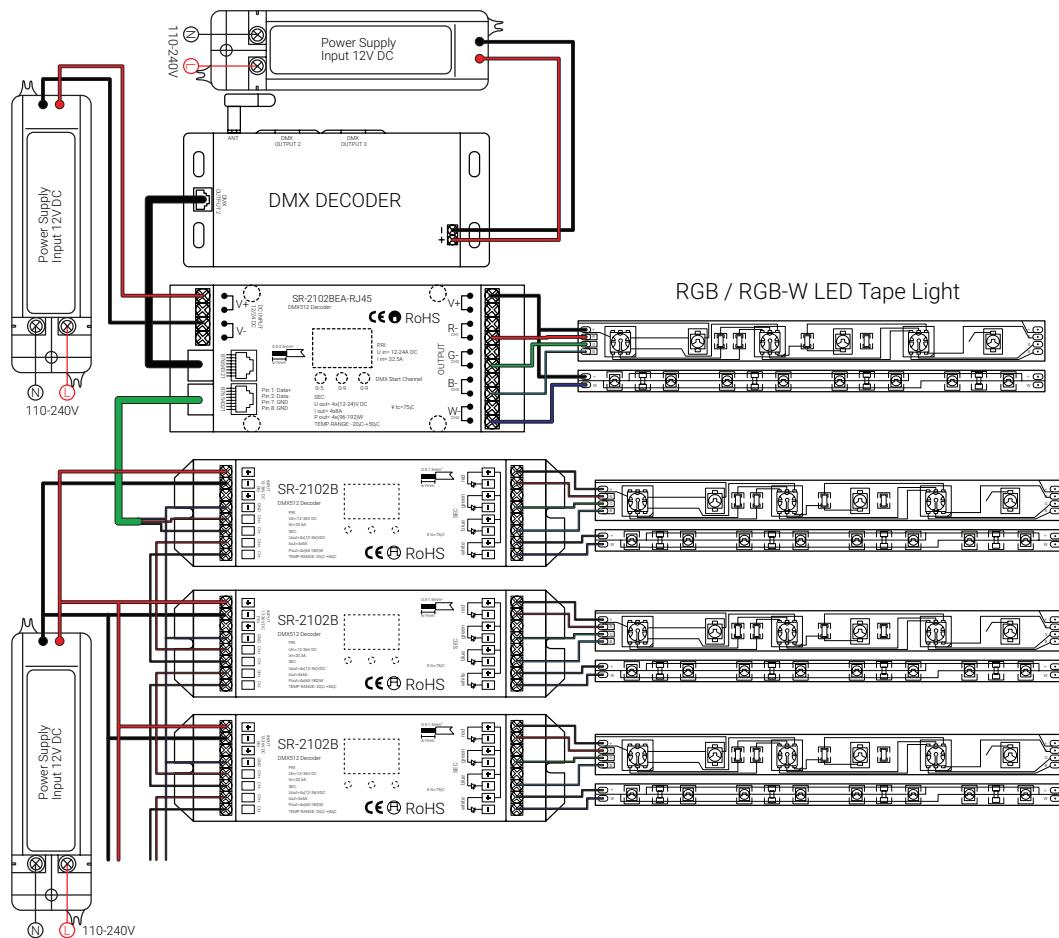
The DMX Decoder translates the digital signals from DMX color controllers, such as the Nicolaudie series, into the analog signal used by Radialux™ RGB and RGB-W 24V LED tape lights. This powerful decoder supports large installations with a clean, consistent signal and is also easy to address with the digital interface.
