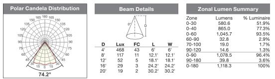
CYL6-1530W: 6" LED CYLINDER, WIDE BEAM SPREAD, 3000 K, 16W
