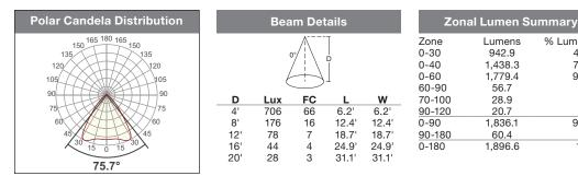
CYL6-3430W: 6" LED CYLINDER, WIDE BEAM SPREAD, 3000 K, 34W
