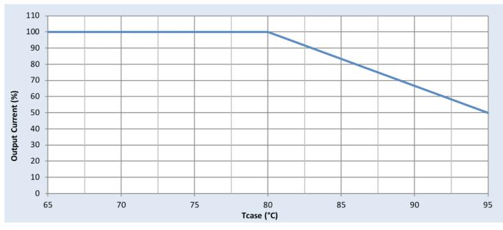
Note: There is  $\pm 5^{\circ}$ C tolerance on the driver case temperature.
