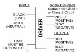
Input and output use lead- wires.
