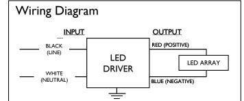
Input and output use lead-wires. Lead-wires are 18AWG 105C/600V solid copper
