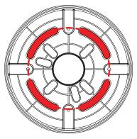
6.5" bolt circle for Drilled Anchors. Used when existing anchor bolts do not fit 4-bolt or 3-bolt slots or are damaged. These must be cut off and new drilled anchors installed.
