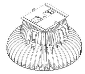
3) Screw the slide piece into the fixture using the bolt and washers provided. The figure below shows the correct orientation.
