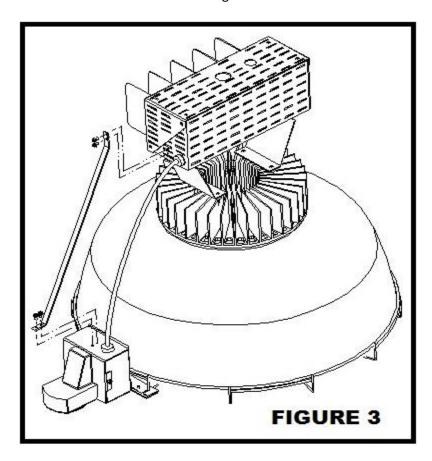
• Make sure that the sensor box is fully secured to the wire cage and driver box. The finished product should closely resemble Figure 4.
