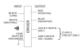
Input and output use lead-wires.
