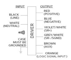
Input and output use lead-wires.
