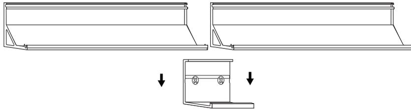
For a 90° corner, slide a channel into each end of the corner connector.
