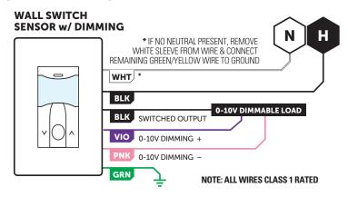
NOTE: This product is UL listed and meets NEC 404.2(c) & 404.22 guidelines regarding powering over ground & current leakage. Powering over ground is permitted for replacement / retrofit only.
