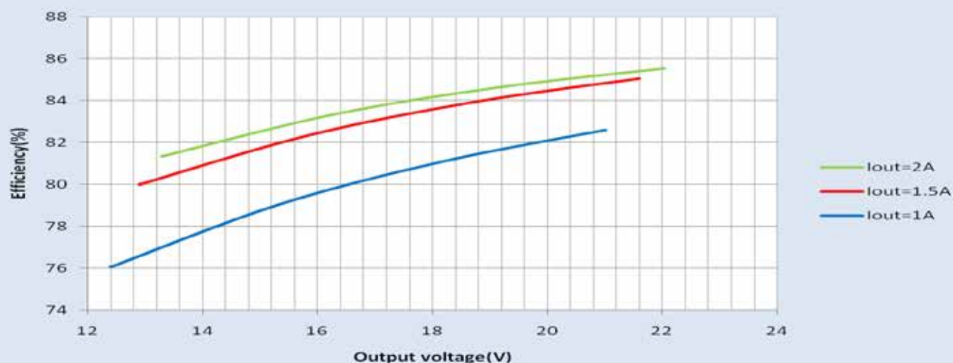
Efficiency Vs. Output Voltage @ 70C TCase and Vin=230 V
