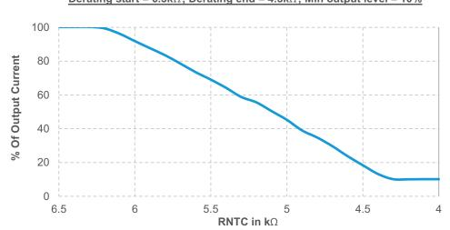
Derating start =  $6.3k\Omega$ ; Derating end =  $4.3k\Omega$ ; Min output level = 10%
