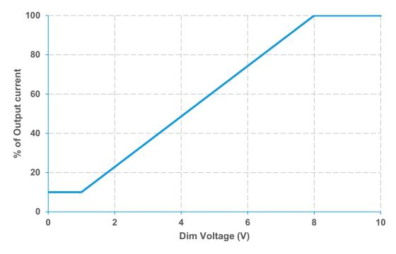
\*The absolute minimum current the driver can deliver is 50mA.
