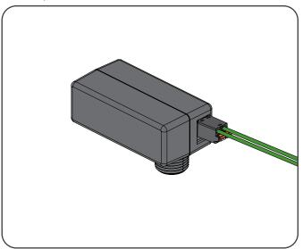
To remove the wires, use a flat head screwdriver to release the wires from the terminal blocks.
