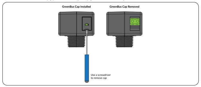
Failure to install black cap for Class 1 wiring schemes may result in exposed hazardous voltages at the GreenBus adapter.
