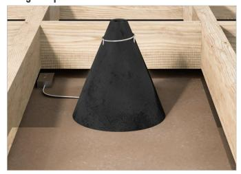
The FF109-250 is a cone-shaped intumescent enclosure which has been specifically designed to help protect openings for **6**<sup>n</sup> low profile LED downlight fixtures. The ultra-flexible nature of the material allows the cover to get rolled up for easy retrofit, remodel or new construction installation from below the ceiling and provide a 60 minute flame, smoke and heat barrier.
